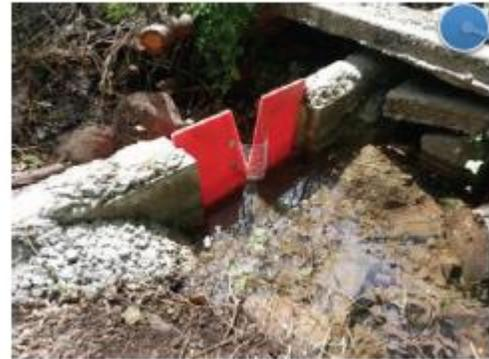
Figure 2 V-notch weir at inlet of study site, 2013
