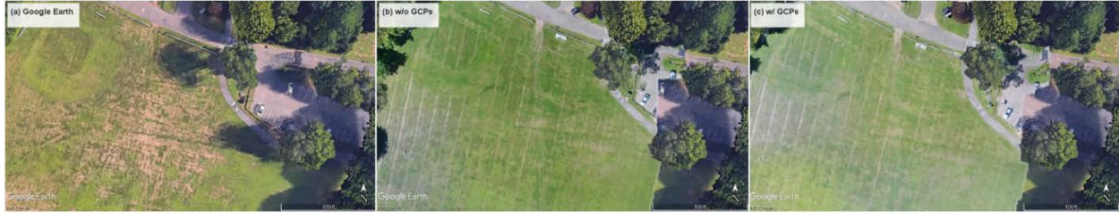
Figure 2. Incorporating GCPs qualitatively improved the accuracy of the orthomosaics when they were overlaid on Google Earth. The (a) Google Earth image is compared to (b) the orthomosaic without GCPs and (c) the orthomosaic with GCPs. Images in (b) and (c) are from Brooksvale Park, Hamden, CT 6/21/17.
