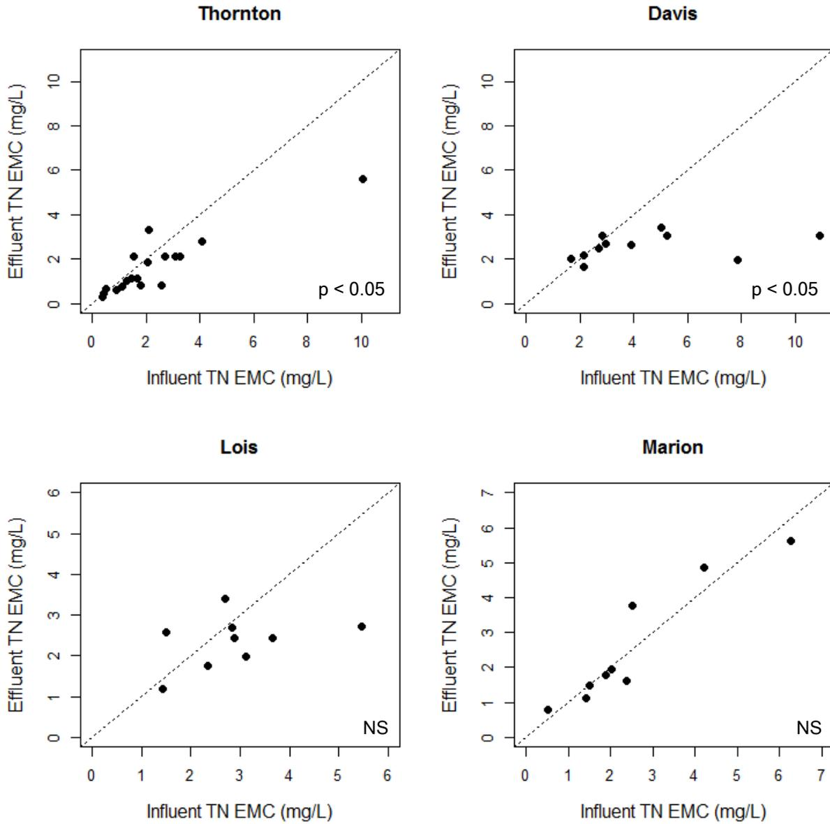
**FIGURE 6.** EFFLUENT TN EMC VS. INFLUENT TN EMC PLOTS FOR EACH WETLAND. DOTTED LINE REPRESENTS  $Y = X$ .
