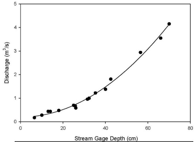
Figure 6: Rating curve relating depth to discharge for the stream gage at the inlet to the West River estuary
