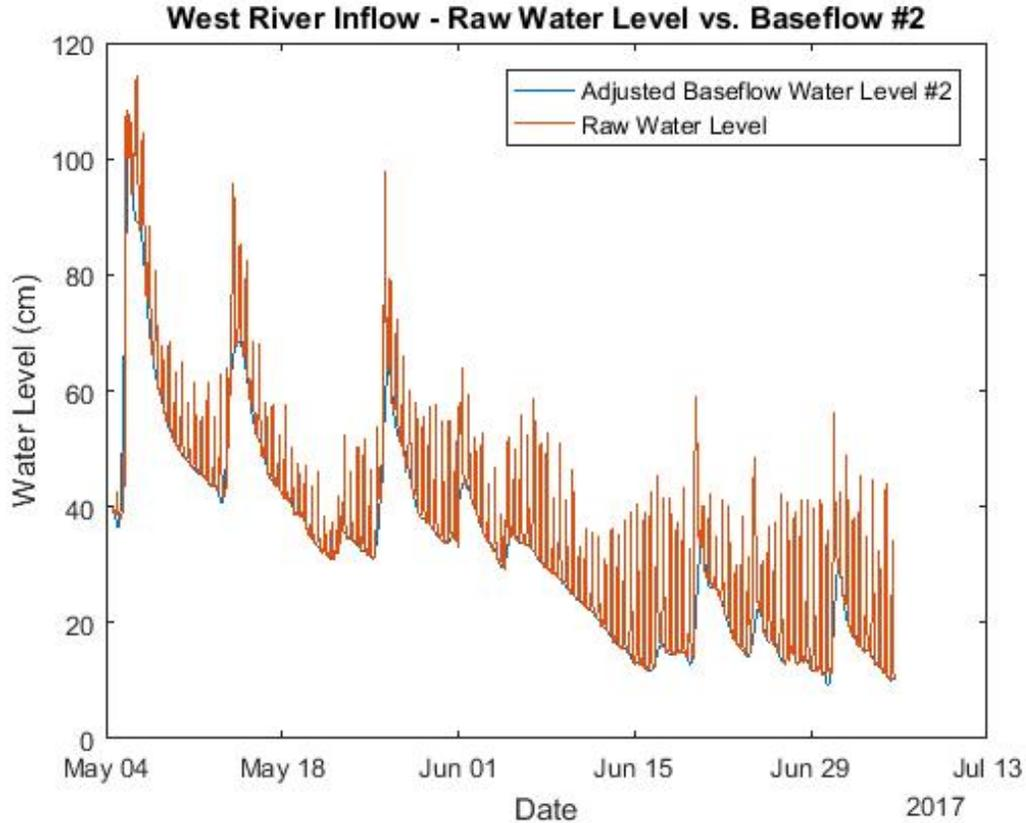
Figure 7: Results of MATLAB program to correct for tidal influence of water depth at inlet
