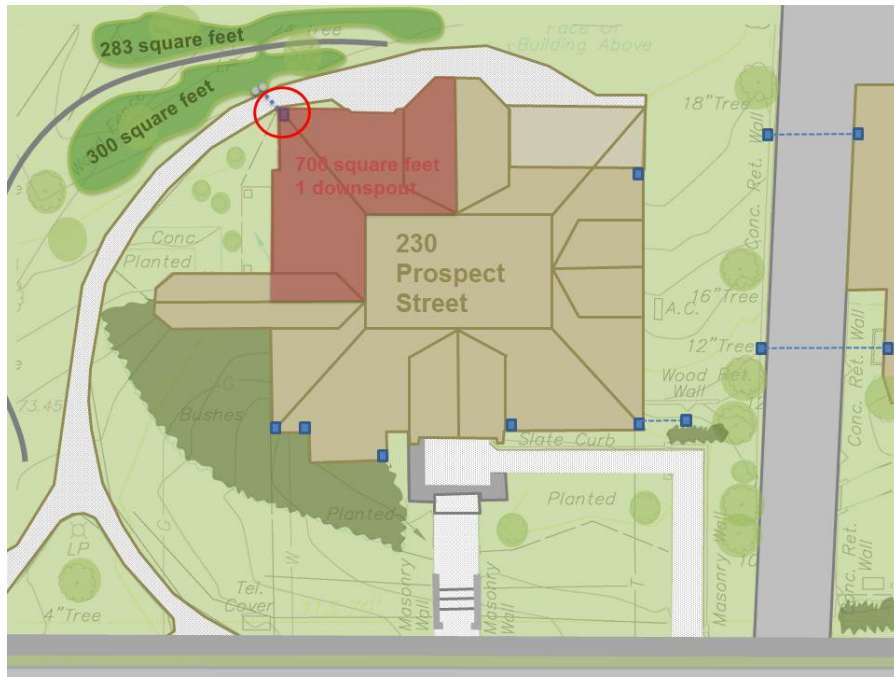
Figure 2: Potential Sizing for Downspout Number 465
