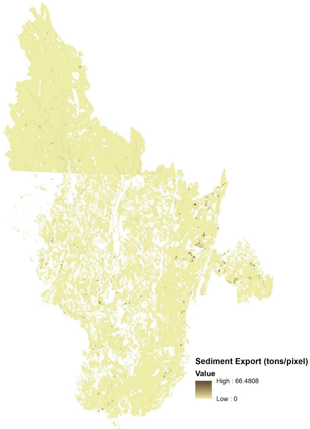
Figure 8. Spatial distribution of annual sediment export in the Farmington watershed for the year 2013. Soil erodibility (K Factor) data was more available in the MA portion of the watershed than the CT portion.
